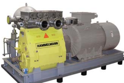
HDP 755 – Reservoir water Op. pressure 212 bar Flow rate 1660 l/min
