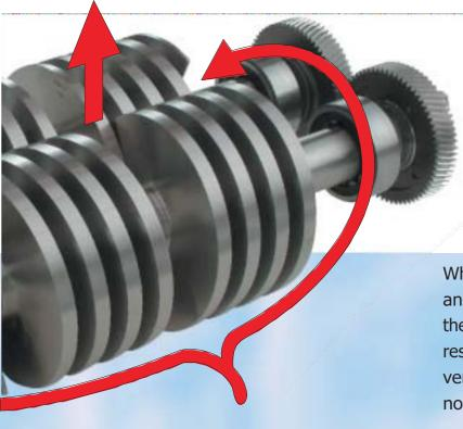
By varying the pitch of the screws the various pressures and flow rates can be achieved.
